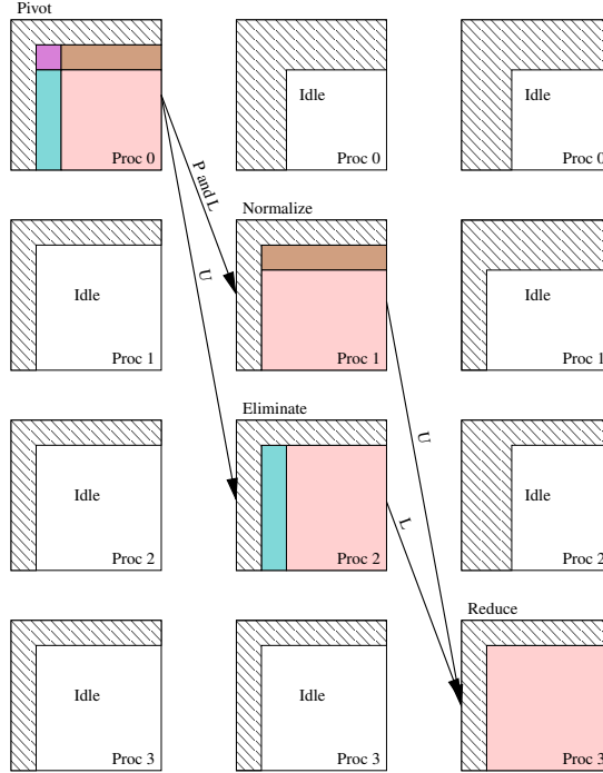
Figure 2: Data send patterns for PLU decomposition using four nodes in the third global pass (corresponds to the situation in Figure 0b). The shaded areas represent the part of the matrix we already have computed.
