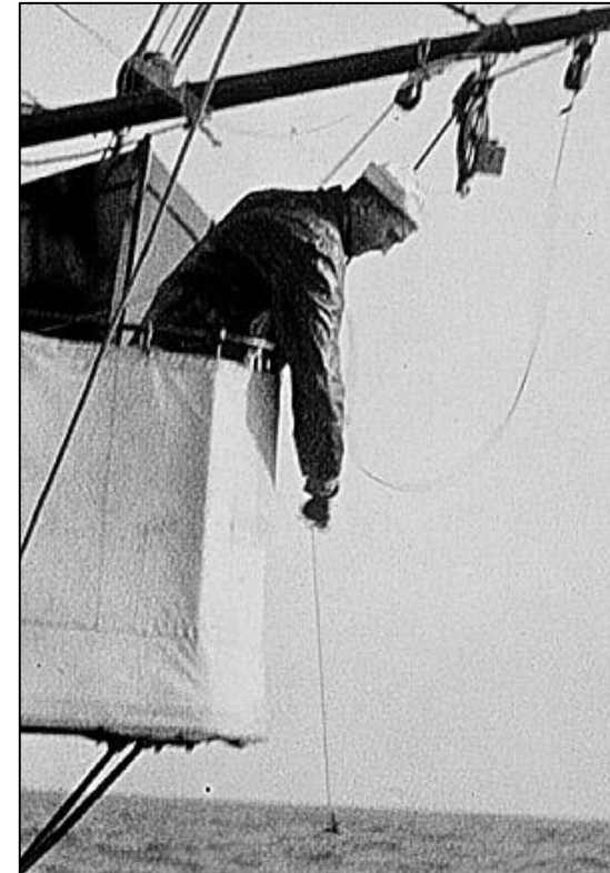
Seaman paying out a sounding line during a hydrographic survey of the East coast of the U.S. in 1916. (NOAA, 2007).
